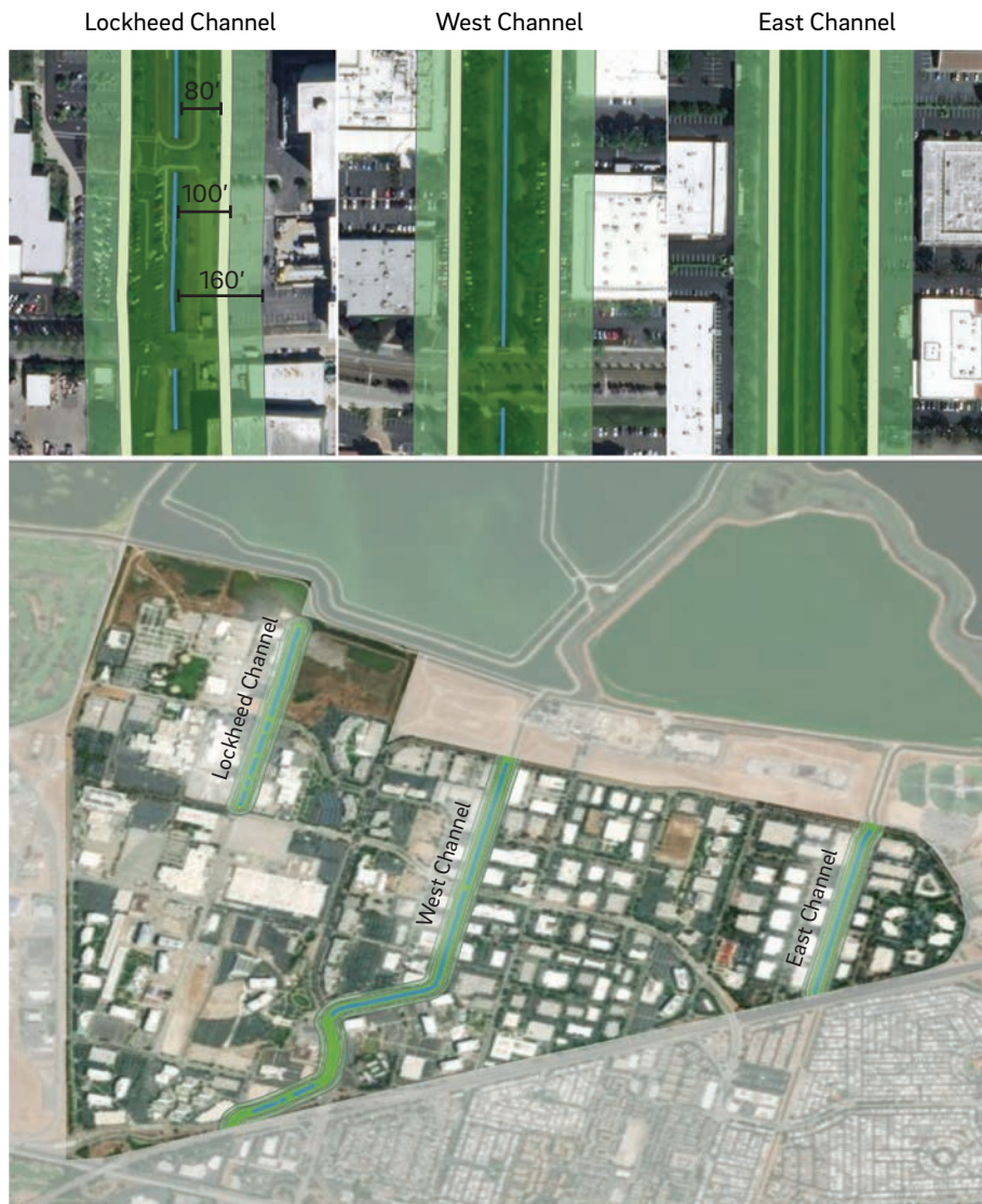
Channel Terrestrial Buffers. Scientifically-based, recommended buffer widths provide different essential functions for riparian areas: (a) 80 feet for pollutant removal, (b) 100 feet for temperature regulation and sediment removal, (c) 160 feet for biodiversity support and bank stabilization. A 330-foot buffer (not shown) is considered optimal for biodiversity.
