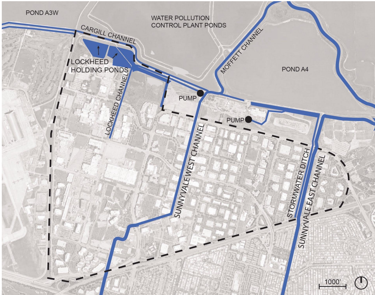
Figure 14. Stormwater channels, pumps, and ponds in Moffett Park (MPSP study area shown with a dashed line).
